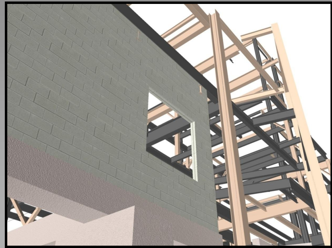
Revit Model of Structural System
